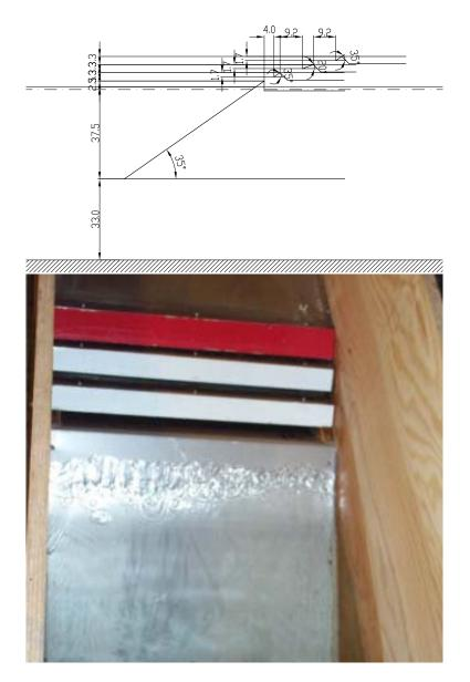
Figure C.12: Drawing (top) and photo (bottom) of model test setup C1, model scale. Measures are in cm.
