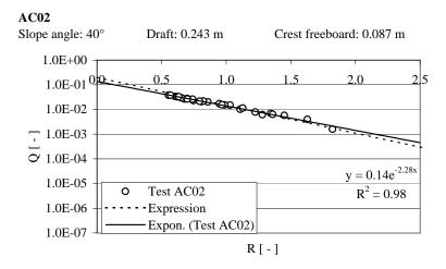
Figure B.11: Results of tests with test geometry AC02.
