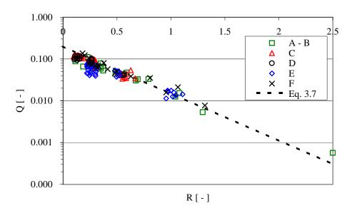
Figure 4.7: Non-dimensionalized total overtopping discharge (sum of all reservoirs) as a function of dimensionless freeboard, compared with eq. 3.10.
