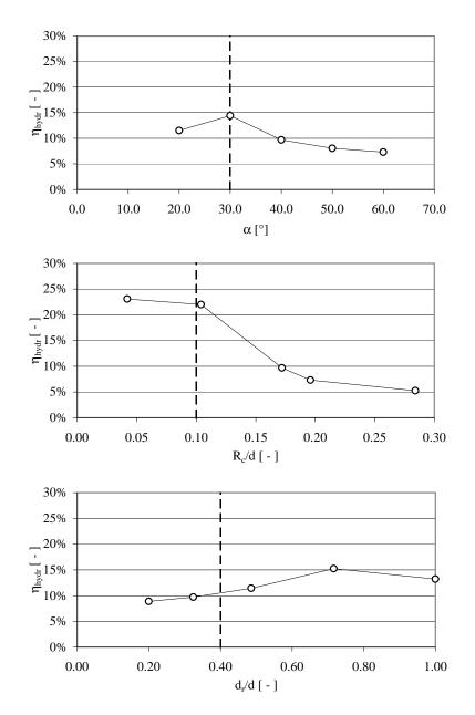
Figure 3.15: The efficiency  $\eta_{hydr}$  of the tested linear slopes plotted as functions of slope angle, relative crest freeboard and relative draft. The vertical broken line indicates the choices for the further model tests.
