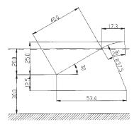
Figure B.21: The geometry of the slope in the CA01 tests. Measures are in cm.
