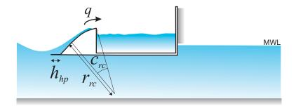
Figure 3.3: Geometrical parameters used for modified slopes.
