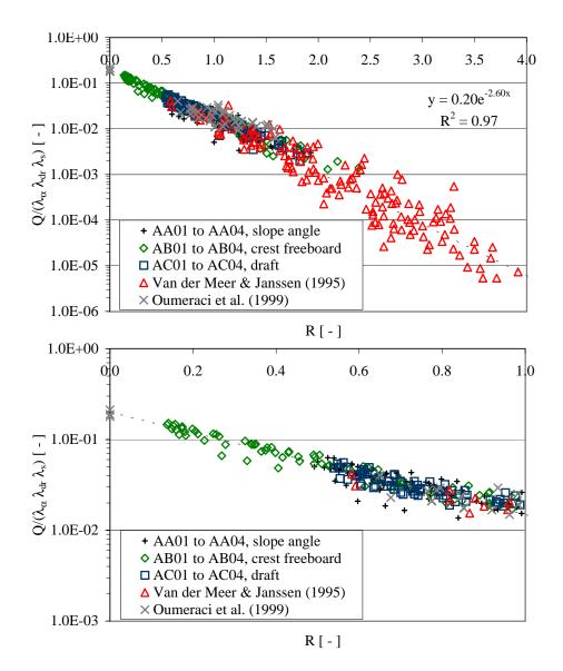
Figure 3.14: The experimental data from the tests with linear slopes plotted together with the overtopping data given in Van der Meer and Janssen 1995 for  $\xi_p > 2$ , and data reported by Oumeraci (1999).  $\lambda_s$  has been introduced. The dotted line represents eq. 2.1. The lower graph is a zoom of the upper graph.
