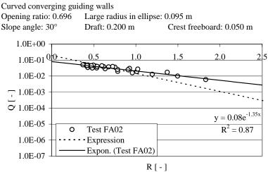
Figure B.39: Results of tests with test geometry FA02.
