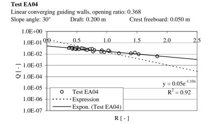
Figure B.37: Results of tests with test geometry EA04.
