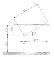
Figure B.19: The geometry of the slope in the BA03 tests. Measures are in cm.
