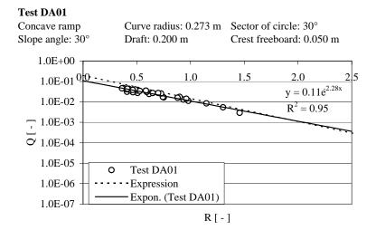
Figure B.32: Results of tests with test geometry DA01.
