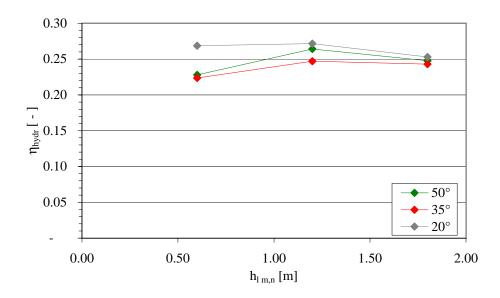
Figure 4.17: Overall hydraulic efficiency  $\eta_{hydr}$  shown as a function of the horizontal opening between the reservoirs  $h_{l,m,n}$ .
