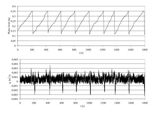
Figure 3.6: An example of a measured water level time series measured in the reservoir (top) and the corresponding time series of the derived overtopping discharge.
