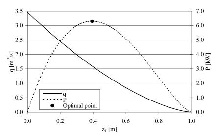
Figure A.2: Plot of overtopping discharge q, and obtained power,  $P(z_1)$ , as a function of the z-level of the string,  $z_1$ .
