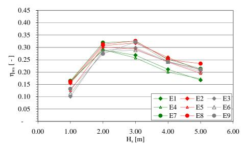
Figure 4.16: Hydraulic efficiency  $\eta_{ws}$  shown as a function of the sea state, characterized by the significant wave height  $H_s$ , for model tests E1 - E9.
