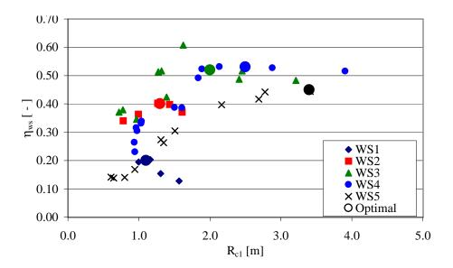
Figure 4.24: Hydraulic efficiency  $\eta_{ws}$  shown as a function of the crest freeboard of the lowest reservoir  $R_{c,1}$  for tests with the floating model. The values of  $R_{c,1}$  considered the optimal for each of the five sea states are marked with large circular dots in corresponding colors.
