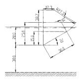
Figure B.31: The geometry of the slope in the DA01 tests. Measures are in cm.
