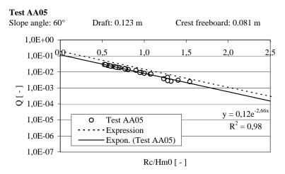
Figure B.5: Results of tests with test geometry AA05.
