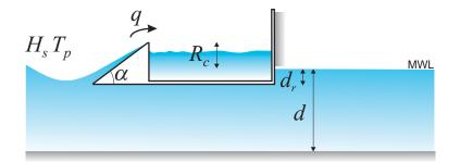
Figure 3.2: Geometric parameters used for linear slopes.
