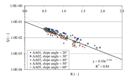
Figure 3.7: Results of tests with test geometries with varying α (test series AA). The dimensionless average overtopping discharge Q is plotted as a function of the dimensionless crest freeboard R. The dotted line represents eq. 2.1 and the solid line is an exponential fit with all the data points shown.
