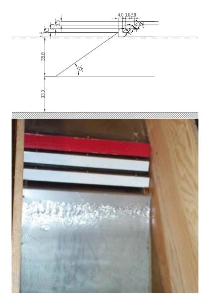
Figure C.11: Drawing (top) and photo (bottom) of model test setup F3, model scale. Measures are in cm.
