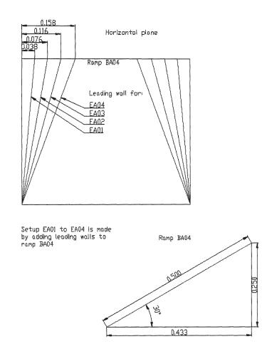
Figure B.33: The geometry of the slope in the EA01 to EA04 tests. Measures are in m.
