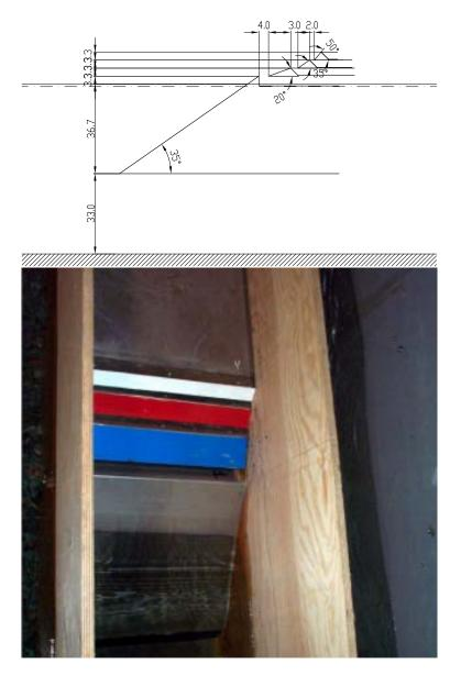
Figure C.10: Drawing (top) and photo (bottom) of model test setup F2, model scale. Measures are in cm.
