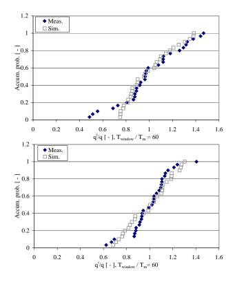
Figure 3.24: Results for the two tests with R = 0.61 (top) and 0.37 (bottom). The accumulated probability density for  $\frac{q_{window}^i}{q}$  is plotted for  $q_{meas}(t)$  and  $q_{sim}(t)$ , respectively.
