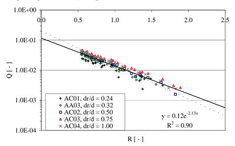
Figure 3.10: Results of tests with test geometries with varying  $d_r$  (test series AC). The dimensionless average overtopping discharge Q is plotted as a function of the dimensionless crest freeboard R. The dotted line represents eq. 2.1 and the solid line is an exponential fit with all the data points shown.
