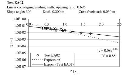
Figure B.35: Results of tests with test geometry EA02.
