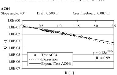
Figure B.13: Results of tests with test geometry AC04.
