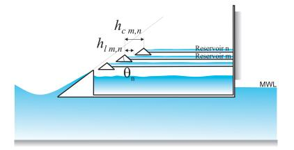
Figure 4.4: Definition of the geometric parameter  $h_{l,m,n}$ , horizontal opening between reservoir m and n, and  $\theta_n$ , angle of the n'th reservoir front.
