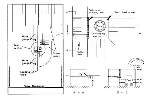
Figure 3.4: Sketch of the model test setup.
