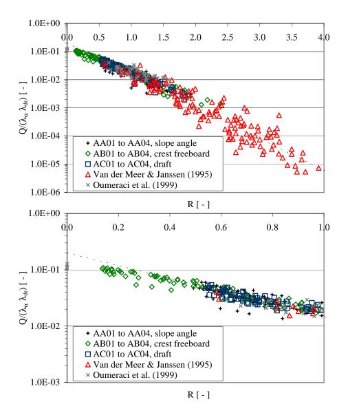
Figure 3.13: The experimental data from the tests with linear slopes plotted together with the overtopping data given in Van der Meer and Janssen 1995 for  $\xi_p > 2$ , and data reported by Oumeraci et al. (1999). The dotted line represents eq. 2.1. The lower graph is a zoom of the upper graph.
