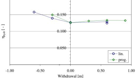
Figure 4.14: Overall hydraulic efficiency  $\eta_{hydr}$  shown as a function of the withdrawal as shown in table 4.2.
