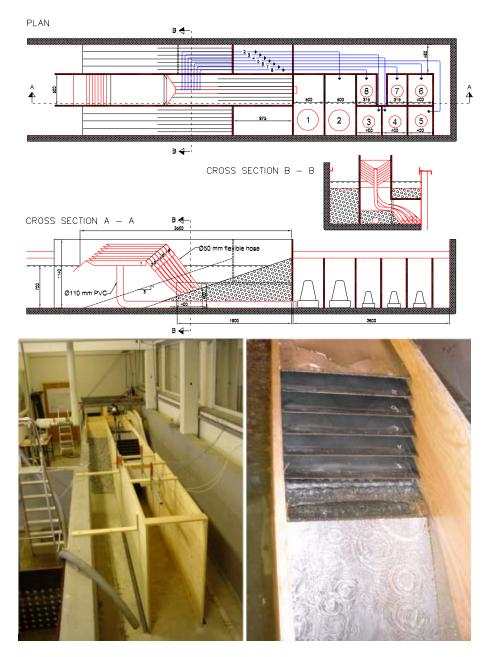
Figure 4.5: Drawings and photos of the model test setup as constructed in the wave flume. Top: Plan view. Middle: Cross section A - A and B - B. Measures are in mm (model scale). Bottom, left: Model test setup before the flume is filled with water. Bottom, right: The model in action.
