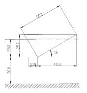
Figure B.15: The geometry of the slope in the BA01 tests. Measures are in cm.
