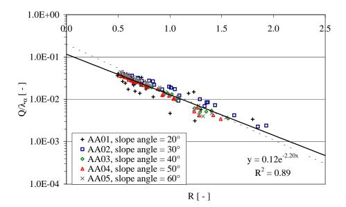
Figure 3.8: Results of tests with test geometries with varying  $\alpha$  (test series AA). The dimensionless average overtopping discharge Q divided by the correction factor  $\lambda_{\alpha}$  is plotted as a function of the dimensionless crest freeboard R. The dotted line represents eq. 2.1 and the solid line is an exponential fit with all the data points shown.
