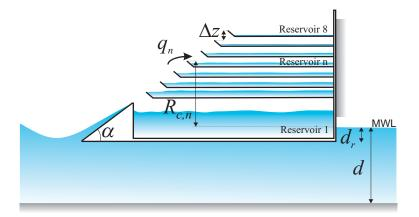
Figure 4.2: Geometric parameters used for multi level reservoirs.
