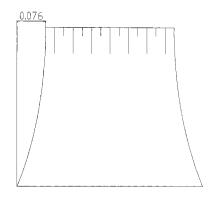
Figure B.38: The shape the of curved converging guiding walls (horizontal projection) for geometry FA02. Measure is in m
