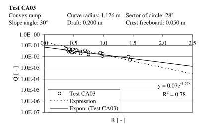
Figure B.26: Results of tests with test geometry CA03.
