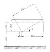
Figure B.17: The geometry of the slope in the BA02 tests. Measures are in cm.
