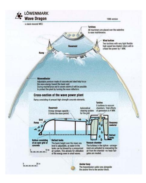
Figure 1.4: Sketch of the working principle of the Wave Dragon. (Illustration by Marstrand.)
