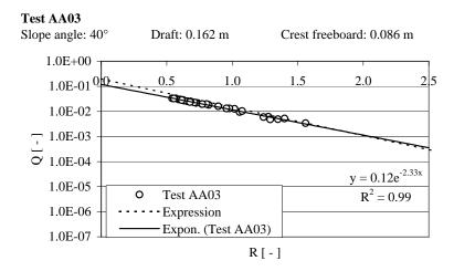
Figure B.3: Results of tests with test geometry AA03.
