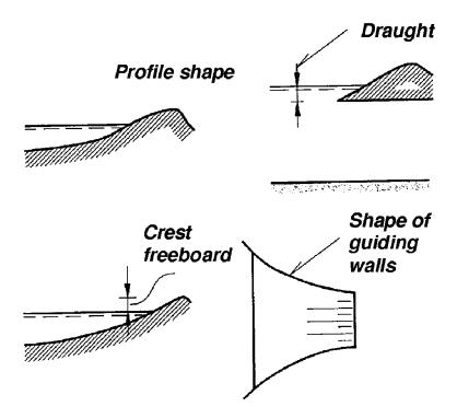
Figure 3.1: Investigated geometric parameters.
