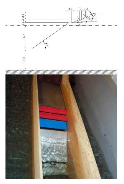
Figure C.9: Drawing (top) and photo (bottom) of model test setup F1, model scale. Measures are in cm.
