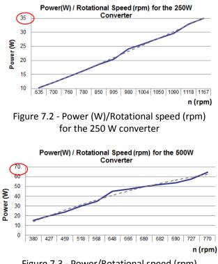
Figure 7.3 - Power/Rotational speed (rpm) for the 500 W converter
