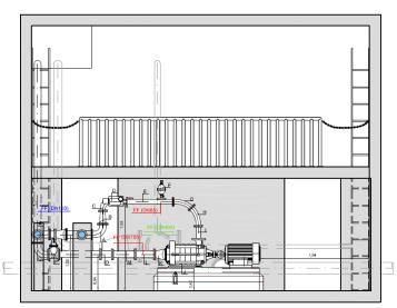
Fig. 8.2 – Installation of PAT (Pump As Turbine) in a reservoir manoeuver chamber
