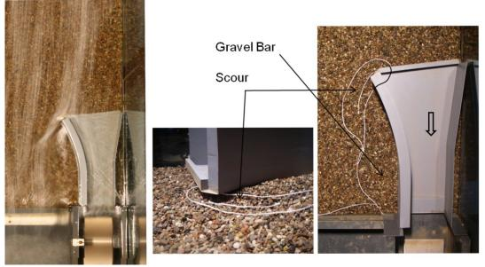
(a) (b) (c) Figure 2a.1: Streamline visualization and bed topography due to an inlet structure.
