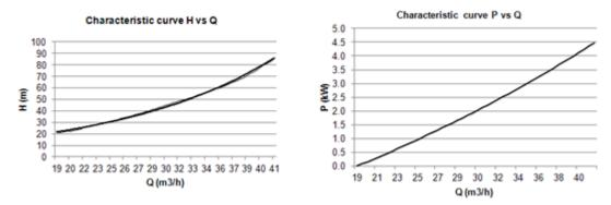
Figure 7.14- PAT characteristic curves obtained Outdoor
