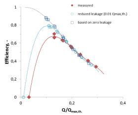
Fig. 2.2: Performance curves of HPM in flume (D = 1200 mm)
