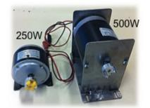
Figure 7.1 - DC permanent-magnet machines
