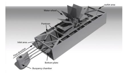
Fig. 5.1: The modelled LSM in CATIA V5
