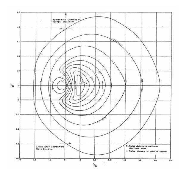
Fig 1.17 Reduction factor for Hs (Ref. SPM, 1984)
