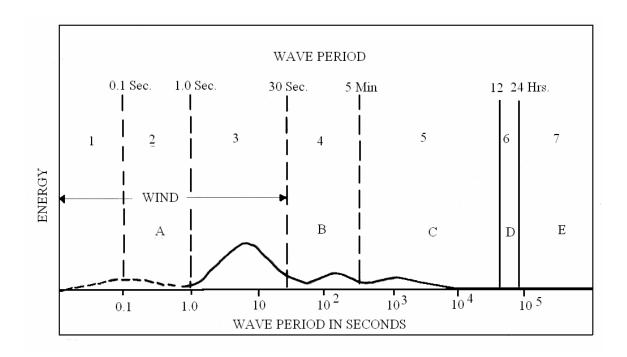
Fig. 1.8 Wave Energy Versus Period (Ref.: Gaythwaite, 1981)
