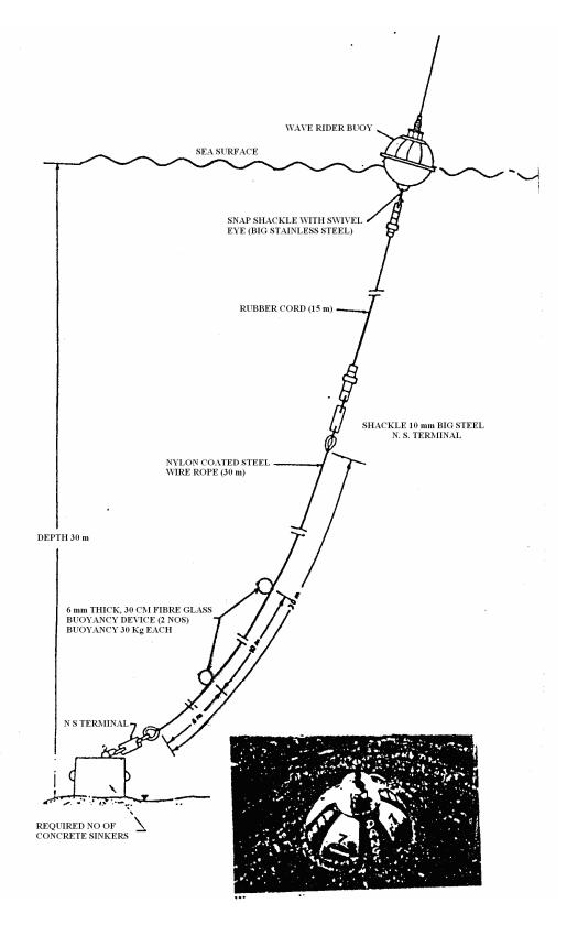
Fig 1.9 Wave Rider Buoy (Ref.: CWPRS, 1993)
