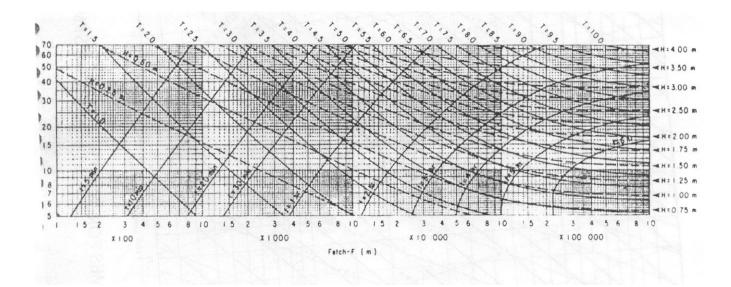
Fig 1.12 SMB Curves for d = 10.5m (**Ref.: SPM, 1984**)
