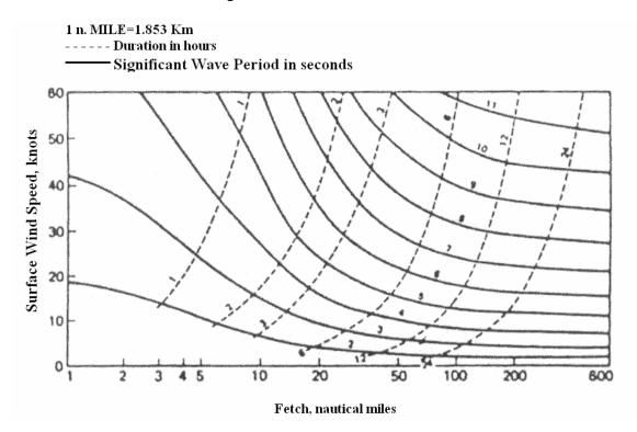
Fig 1.15 b T<sub>s</sub> for Coastal Waters (Ref. Brebbia and Walker, 1979)
