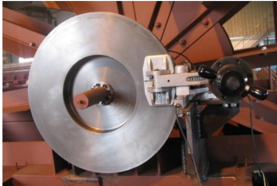
(b) Disk break and callipers instrumented with load-cell
