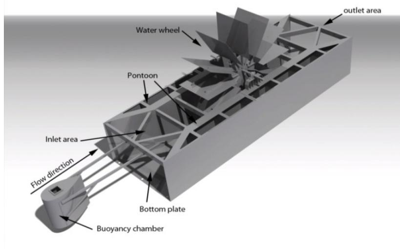
Fig. 5.1: The modelled LSM in CATIA V5
