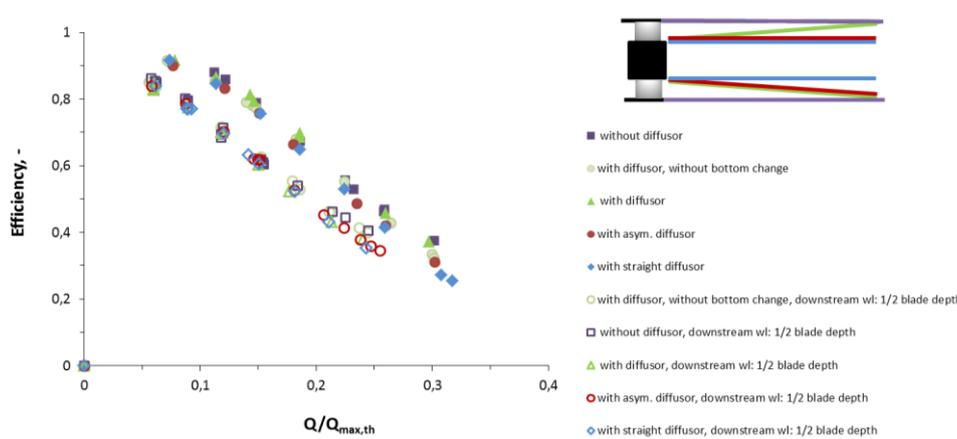
Fig. 2.3: Performance curves for different downstream water levels and different diffusors
