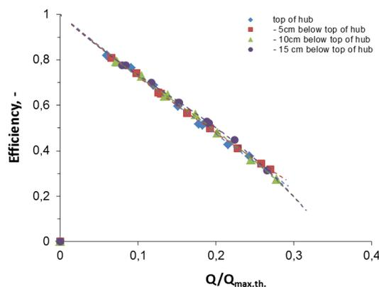
Fig. 2.4: Performance curves for different upstream water levels
