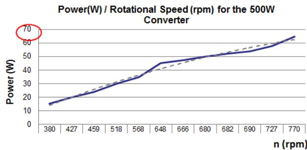
Figure 7.3 - Power/Rotational speed (rpm) for the 500 W converter
