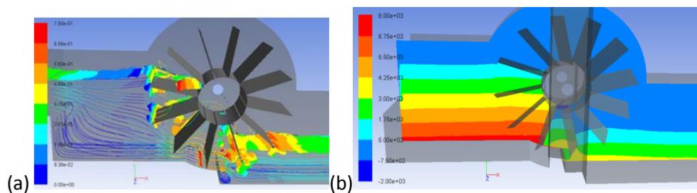
Fig. 9.1: Velocity contour (a) and pressure distribution
