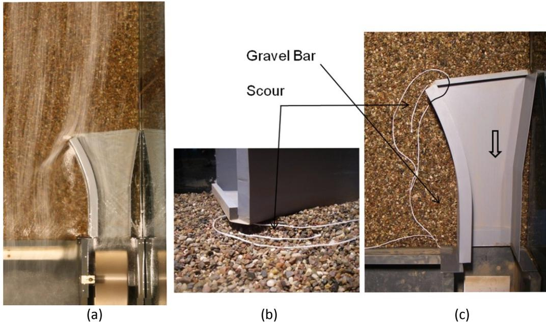
Figure 2a.1: Streamline visualization and bed topography due to an inlet structure.
