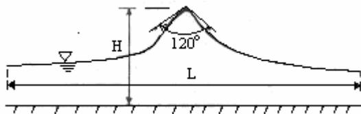
Fig 1.6 Wave Breaking
