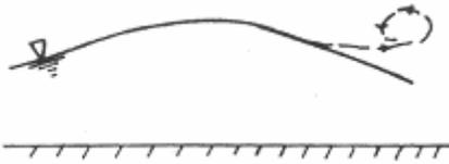
Fig 1.2 Flow Separation At Crest
