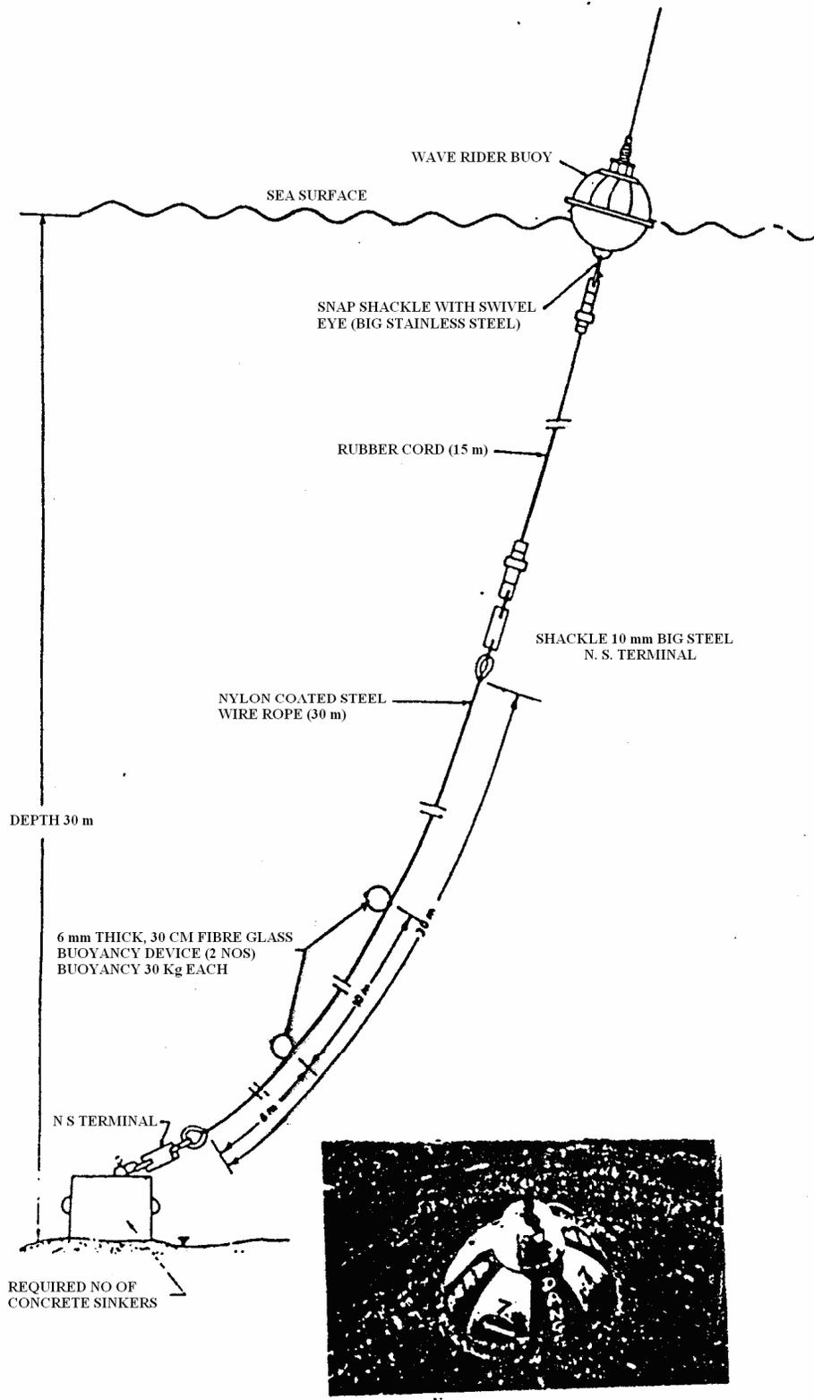
Fig 1.9 Wave Rider Buoy (Ref.: CWPRS, 1993)
