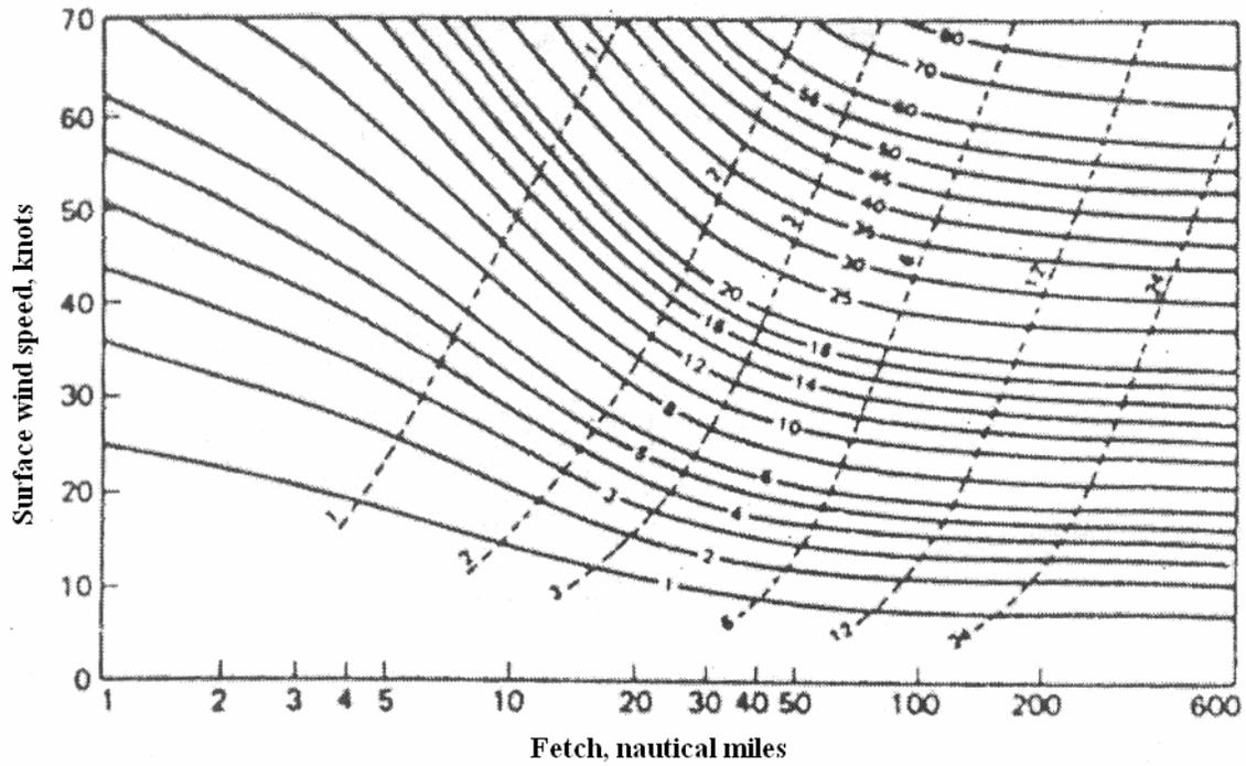
Fig 1.16 a  $H_{10}$  for Oceanic Waters
