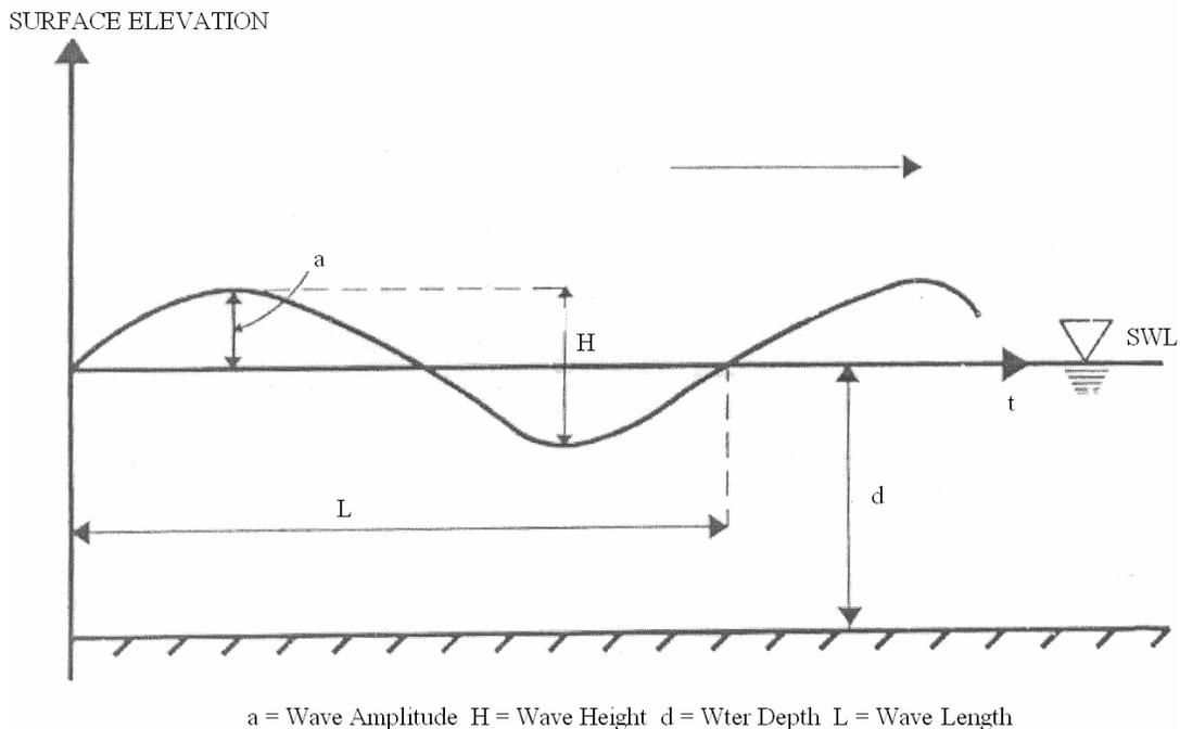
Fig 1.1 Definition Sketch Of a Propagating Wave
